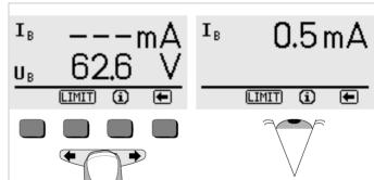
If the START key is press and held, I<sub>B</sub> is measured and displayed.
