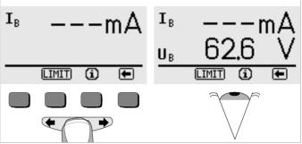
$\, \diamond \,\,$  Briefly press the START key in order to start the measurement. Contact voltage  ${\rm U}_{\rm B}$  is measured and displayed.
