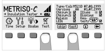
The self-test is started from the main menu with the Test key. The test has a duration of several seconds.
