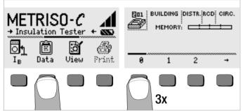
Enter memory address "000". After acknowledgement by pressing button START (press at center) a safety request appears.
