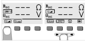
Select the U\_function from the U<sub>ISO</sub> menu with the or the key and acknowledge with the U\_key.
