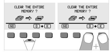
By simultaneously activating O and K all data that have been saved are deleted from memory. The bar graph to the right of the parameter "MEMORY:" is empty. To the left, memory address "001" is displayed. New data can now be entered for the first address, or the database can be exited (press J or START 9 times).
