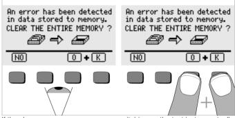
If the above message appears upon switching on the test instrument, all data can be saved to a PC before finally deleting the database in order to rectify the error.
