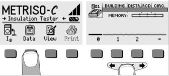
Acknowledge with the START key (press at center). All data from the selected memory address are deleted.
