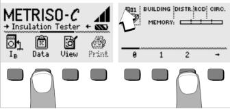
First create the desired memory address with the help of the softkeys. After acknowledging with the START key (press at center), the cursor appears at the first data entry position (BUILDING). With the help of the softkeys, entries can be made to the BUILDING, DISTRIBUTOR CABINET, RCD No. and CIRCUIT fields one after the other, and a designation can be entered for the electrical circuit.
